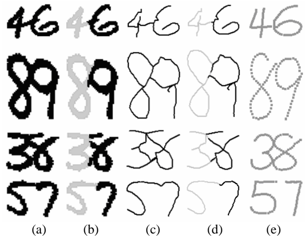
Figure 7. Examples of segmentation results: (a) normalized input images; (b) the segmentation results on the input image; (c) normalized skeletons of input images; (d) segmentation results on the skeletons; (e) numeral pair models generated for the recognition result.
